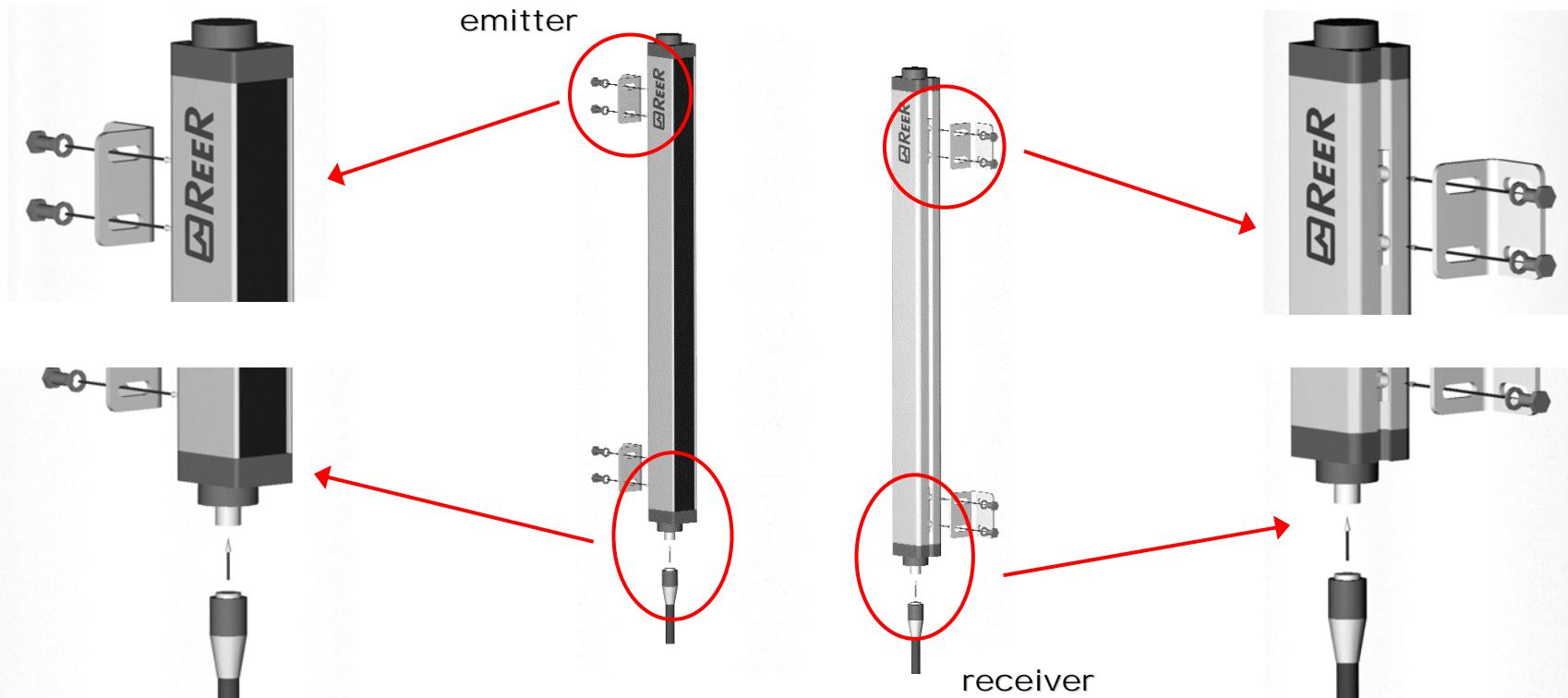
**B) OPTICAL ALIGNMENT - ALLINEAMENTO OTTICO - ALIGNEMENT OPTIQUE - OPTISCHE AUSRICHTUNG - ALINEAMIENTO ÓPTICO - OPTISCHE UITLIJNING**
